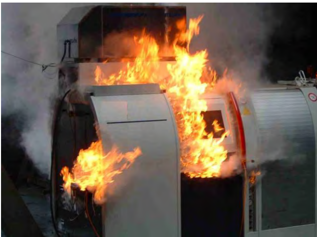
Figure 1: Flame ejection in the door area at the ignition of the MWF/oil-air mixture in the machining room
