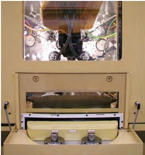
Figure 7: Loading and unloading station of raw and finished parts on a multispindle automatic lathe
